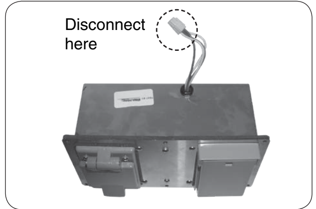
Fig. 37-2 Slightly pull out box and disconnect wire harness
